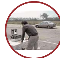
Pass-by Noise test
